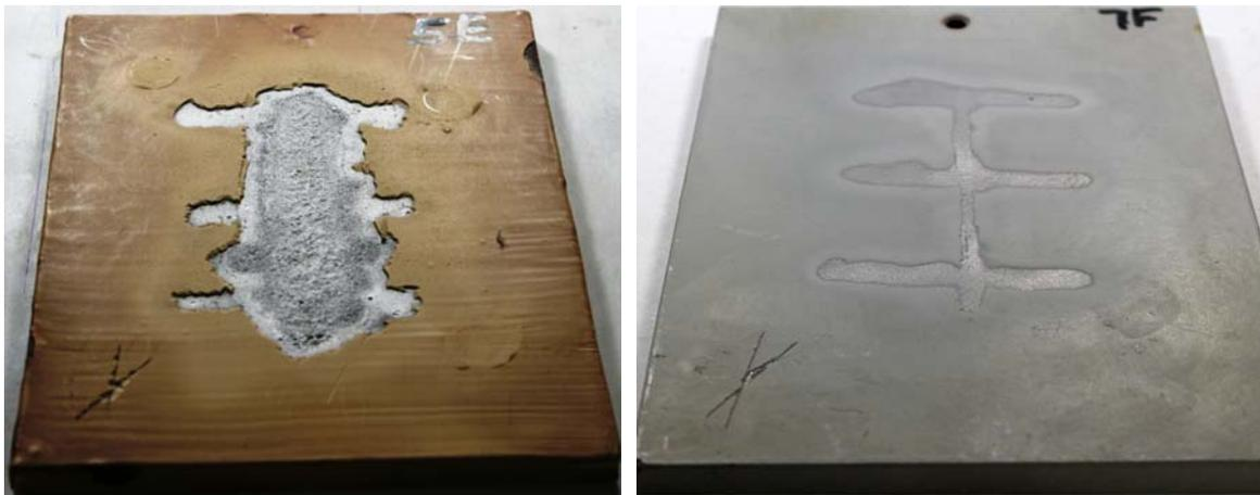
**Figure 13. Pitting under system 5 (left) and 7 (right) after cleaning.**
