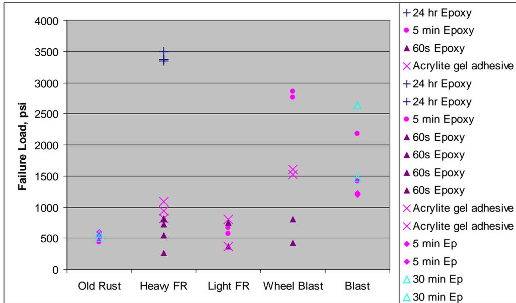
Figure 9. Preliminary pull-off adhesion data.
