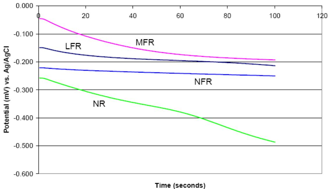
Figure 4. Potential vs time relationship of flash rusted panels from Reference ii. NR = No Rust (mechanically abraded); NFR = No Flash Rust; LFR = Light Flash Rust; MFR = Moderate Flash Rust.
