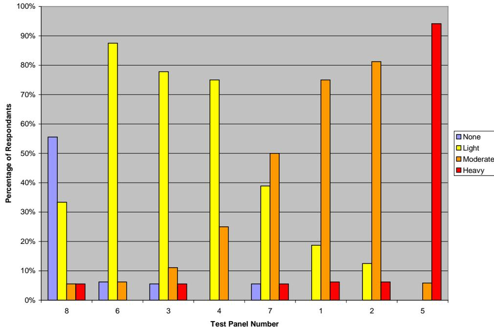
**Figure 1. Flash Rust Ratings Provided by Multiple Inspectors during Round Robin**
