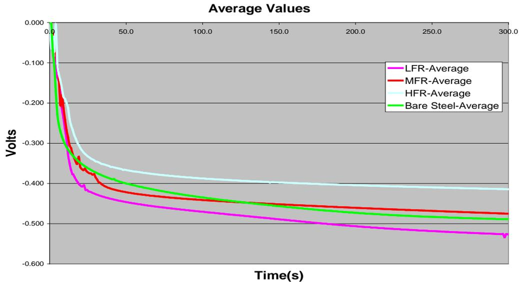
Figure 5. Potential vs time relationship of flash rusted panels from Reference viii.
