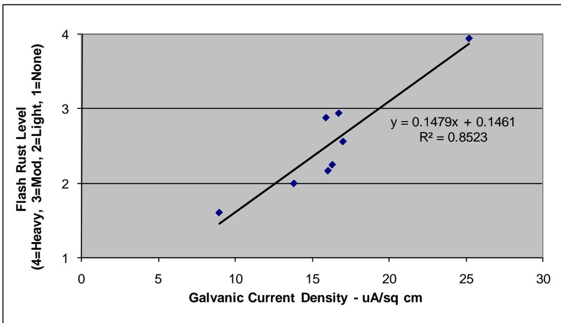
Figure 8. Correlation between Galvanic Current Density and Flash Rust Rating
