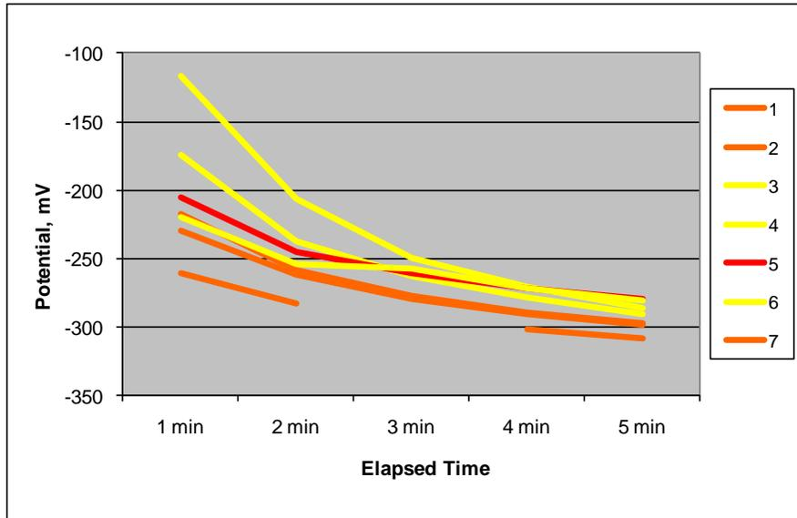
**Figure 6. Potential vs time relationship of flash rusted panels from NSRP study. The line colors correspond to the flash rust condition: red = heavy, orange = moderate, yellow = light.**
