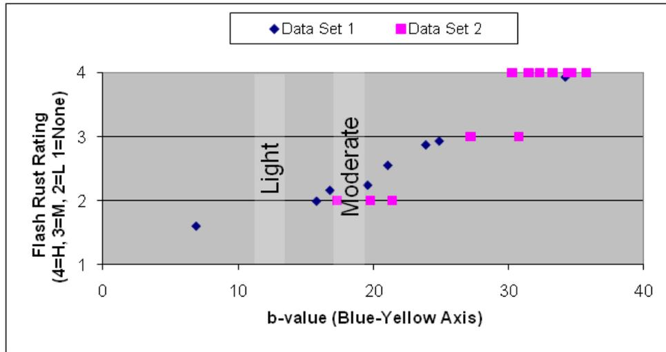
Figure 3. Colorimeter data from varying flash rust panels.
